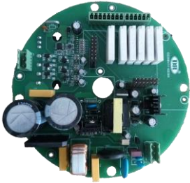
电源板/Power panel
