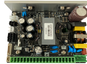
Fig.11: Independent power supply module
