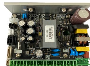
Fig.12: Independent power supply module
